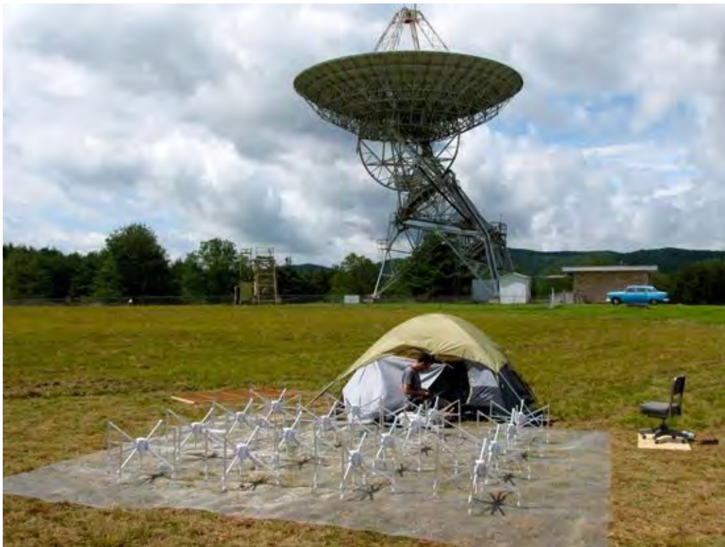
Figure 4.8: Radio astronomy on a big (background) and small (foreground) budget. My grad student Andy Lutomirski is tinkering with our electronics unit, which we put in a tent for rain protection during our expedition to Green Bank, West Virginia.
